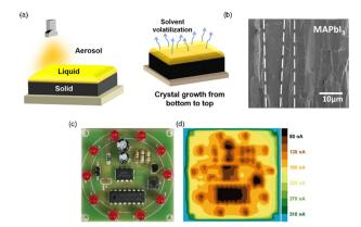
Fig. 6 Spray coating method. (a) The schematic diagram of spray coating. (b) Cross sectional SEM image of the MAPbI<sub>3</sub> film by spray coating. Reproduced with permission. 104 Copyright 2021, Elsevier. (c) Photograph of a circuit. (d) X-ray imaging of the circuit by the 2D (PEA)<sub>2</sub>MA<sub>3</sub>Pb<sub>4</sub>I<sub>13</sub>/3D MAPbl<sub>3</sub> detector.<sup>56</sup>
