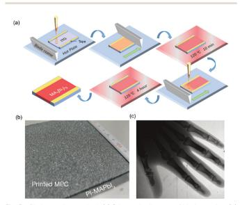
Fig. 5 Blade coating method. (a) Schematic diagram of blade coating. (b) Printed MAPbI<sub>3</sub> film.<sup>80</sup> (c) Hand skeleton image by the MAPbI<sub>3</sub> detector. Reproduced with permission.<sup>63</sup> Copyright 2017, Springer Nature.
