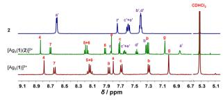
Fig. 1 Partial <sup>1</sup>H NMR (600 MHz,  $CD_2Cl_2$ , 298 K) of silver(i)-loaded deck  $[Aq_3(\mathbf{1})]^{3+}$ , slider-on-deck  $[Aq_3(\mathbf{1})(2)]^{3+}$  and biped **2**.
