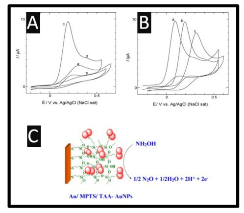
Fig. 1 (A) Cyclic voltammograms obtained for 0.50 mM hydroxylamine at (a) bare Au, (b) Au/MPTS, (c) Au/MPTS/TAA-AuNPs modified electrodes in 0.2 M PB solution (pH = 7.2) at a scan rate of 50 mV s<sup>-1</sup>. (B) Cyclic voltammograms obtained for 0.50 mM hydroxylamine in 0.2 M PB solution (pH = 7.2) at a pH of 9.2 (a), 7.2 (b) and 5.2 (c). (C) An overview of the mechanism. Reprinted with permission from ref. 13. Copyright 2010 Elsevier.
