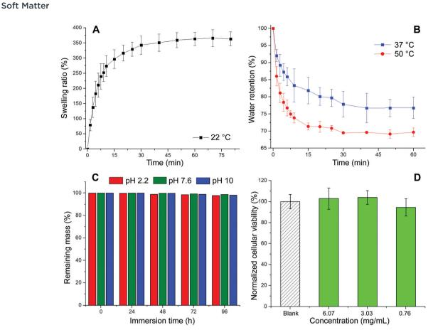
Fig. 3 (A) Evolution of swelling ratio and (B) water retention parameters as a function of time in PBS buffer solution. (C) Hydrogel stability over time measured at different pH values. (D) Cell-viability assay.
