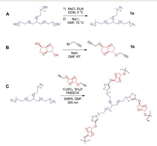
Scheme 1 Synthetic protocols employed in the preparation of (A) triazide glycerol ethoxylate and (B) bis-alkyne isosorbide derivates. (C) Synthesis of hydrogel films via Cu(i) mediated photo-click reaction
