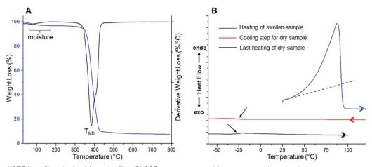
Fig. 2 (A) TGA and DTGA profiles obtained for a dry film. (B) DSC curves measured for a water-swollen sample
