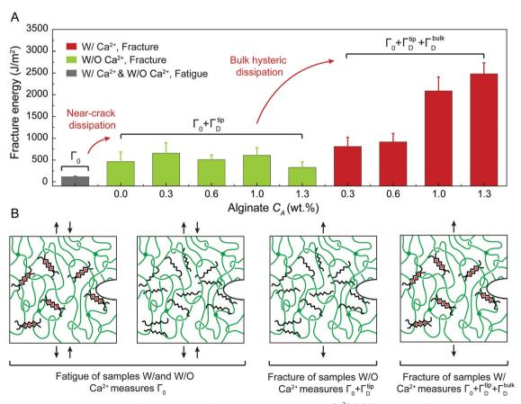
Fig. 4 Summarized fracture toughness and fatigue threshold of hydrogels with and without Ca<sup>2+</sup>. (A) Three levels of fracture energies of the two series of PAAm-alginate hydrogels. (B) Schematic illustration of fatigue test of hydrogels with and without  $Ca^{2+}$  measuring  $\Gamma_0$ , fracture test of hydrogels without  $Ca^{2+}$  measuring  $\Gamma_0 + \Gamma_D^{tip}$ , and fracture test of hydrogels with  $Ca^{2+}$  measuring  $\Gamma_0 + \Gamma_D^{tip} + \Gamma_D^{tip}$ .
