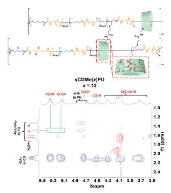
Fig. 2 600 MHz 2D NOESY NMR spectrum of γCDMe(13)PU in chloroform-d. The NOE correlation signals between the TAcγCD units and the PU main chains are highlighted.
