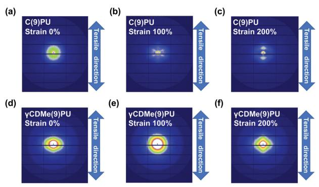
Fig. 6 2D small-angle X-ray scattering (SAXS) patterns of (a-c) C(9)PU and (d-f) γCDMe(9)PU with 0%, 100% and 200% strain. The direction of tensile testing is shown by the arrow.
