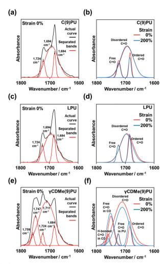
Fig. 5 Actual FT-IR spectra and separated bands after peak deconvolution of C(9)PU (a), LPU (c), and γCDMe(9)PU (e) before tensile stretching. Changes in the separated bands of C(9)PU (b), LPU (d), and  $\gamma$ CDMe(9)PU (f) during tensile stretching from 0% to 200% strain.
