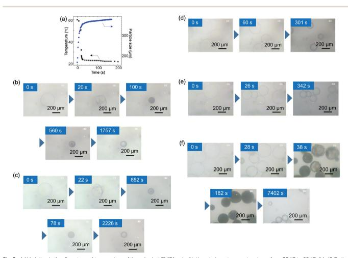
Fig. 8 (a) Variation in the diameter and temperature of the spherical PNIPA gel with time during a temperature jump from 20 °C to 60 °C, (b) – (f) Optical microscopy images in a temperature jump from 60 °C to 20 °C for (b) PNIPA gel, (c) PNIPA<sub>0.9</sub>-b-PDMA<sub>0.1</sub> gel, (d) PNIPA<sub>0.8</sub>-b-PDMA<sub>0.2</sub> gel, (e) PNIPA<sub>0.7</sub>-b-PDMA<sub>0.3</sub> gel, and (f) PNIPA<sub>0.8</sub>-r-PDMA<sub>0.2</sub> gel.
