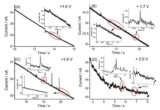
Fig. 3 (A)-(D) Examples of representative chronoamperometric profiles of nano-impact at different potentials (1.60, 1.70, 1.80 and 2.00) in a 0.1 M KNO<sub>3</sub> (pH = 6.4) solution containing 0.01 g  $L^{-1}$  MWCNTs. No spikes or steps were detected below/at 1.50 V.
