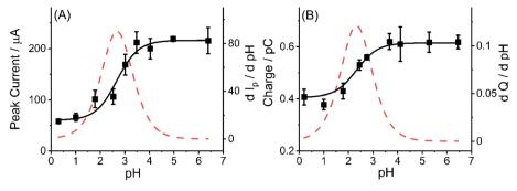
Fig. 8 (A) Relationship between oxidative peak current of MWCNTs-NH<sub>2</sub> modified GCE and pH value of solution; (B) relationship between average charge of oxidative spikes and pH value of solutions in the presence MWCNTs-NH2 (black square: experimental data; black solid line: simulated curve, and red dotted line: differential curve of experimental data).
