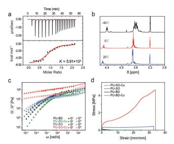
Fig. 2 (a) The ITC titration data of the SO ligand with CuCl<sub>2</sub> in anhydrous MeOH at 298 K. (b) Variable-temperature <sup>1</sup>H nuclear magnetic resonance (<sup>1</sup>H NMR) for PU-SO-Cu. (c) Master curves of PU-BD, PU-BD-Cu, PU-SO and PU-SO-Cu scaled by time-temperature superposition (TTS) at a reference temperature of 20 °C. (d) Typical stress-strain curves of different samples including PU-BD, PU-BD-Cu, PU-SO and PU-SO-Cu, with a strain rate of 20 mm min<sup>-1</sup>
