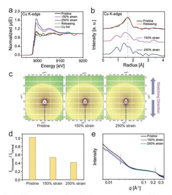
**Fig. 4** (a) XANES spectra of PU–SO–Cu under different strains. (b) EXAFS spectra of PU–SO–Cu under different strains. (c) 2D SAXS images of PU–SO–Cu with different extension strains during the uniaxial stretching process. (d) Ratio of intensities integrated in different directions (horizontal and vertical) under different strains. All intensities were calculated at  $q=0.024~\text{Å}^{-1}$ . (e) 1D scattering profiles of PU–SO–Cu integrated from 2D SAXS patterns under different strains.
