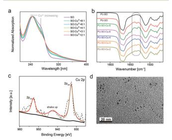
Fig. 1 Structural characterization studies of the PU-SO-Cu elastomer. (a) UV-Vis spectra of samples with different SO: Cu<sup>2+</sup> ratios in MeOH. The curves were normalized using the absorption band at about 250 nm. (b) FT-IR spectra of different samples. (c) The XPS spectrum of the Cu 2p region in PU-SO-Cu. (d) TEM image of a dynamic interaction system in the PU-SO-Cu substrate. Scale bar: 20 nm.
