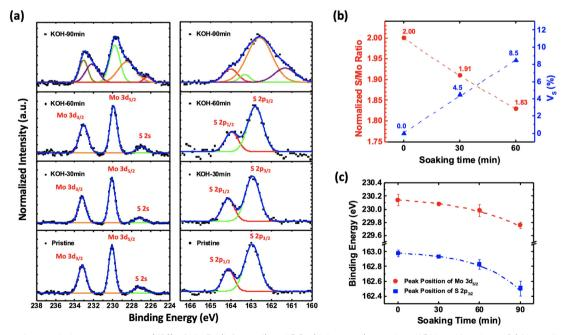
Fig. 2 (a) X-ray photoemission spectroscopy (XPS) of Mo 3d (left panel) and S 2p (right panel) at various KOH soaking times. (b) Normalized S/Mo ratio and S-vacancy ( $V_S$ ) as a function of soaking time showing an increasing percentage of  $V_S$  with increasing soaking time. (c) Peak positions of Mo  $3d_{5/2}$  and S 2p<sub>3/2</sub> shift to lower binding energy values with increasing soaking time.
