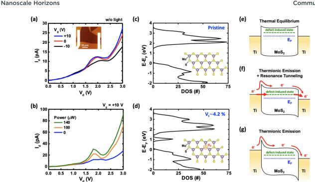
Fig. 4 (a)  $I_d - V_d$  curves at different gate voltages without light illumination. The inset presents the OM image of the measured device. (b)  $I_d - V_d$  curves illuminated with different light power values at a fixed gate voltage  $V_0 = +10 \text{ V}$ . (c and d) Density of states (DOS) of pristine monolayer MoS<sub>2</sub> and that with  $V_{\rm S} \approx 4.2\%$ , respectively. (e-g) Schematics of band diagrams for different stages of the NDR mechanism.
