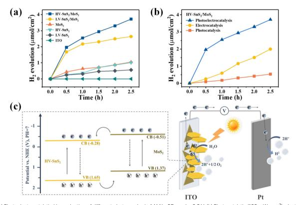
Fig. 9 (a) Photoelectrocatalytic  $H_2$  production of different photoanodes in 1 M  $H_2SO_4$  under 0.8 V. (b) Photocatalytic (100 mW cm $^{-2}$ ), electrocatalytic (0.8 V), and photoelectrocatalytic (100 mW cm $^{-2}$ , 0.8 V)  $H_2$  production of HV-SnS $_2/MoS_2$  photoanode. (c) The schematic plot of charge transfer pathways in HV-SnS $_2/MoS_2$  heterostructure as an effective photoelectrode for PEC water splitting.
