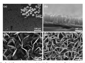
Fig. 2 (a) Top optical image of the MoS<sub>2</sub> nanosheets. The inset is a high magnification optical image. (b) Sectional-view SEM image of HV-SnS<sub>2</sub>. (c) Top SEM image of LV-SnS<sub>2</sub>/MoS<sub>2</sub>. (d) Top SEM image of HV-SnS<sub>2</sub>/MoS<sub>2</sub>.
