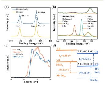
Fig. 4 (a) XPS spectra of Sn  $3d_{3/2}$  and Sn  $3d_{5/2}$ . (b) XPS spectra of Mo  $3d_{3/2}$ and Mo 3d<sub>5/2</sub>. (c) VB spectra and VBM fitting of HV-SnS<sub>2</sub> and MoS<sub>2</sub>. (d) Band alignment information of HV-SnS<sub>2</sub>/MoS<sub>2</sub>
