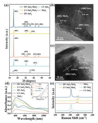
Fig. 3 (a) XRD pattern of HV-SnS<sub>2</sub>/MoS<sub>2</sub>, LV-SnS<sub>2</sub>/MoS<sub>2</sub>, HV-SnS<sub>2</sub>, LV- $SnS_2$ , and  $MoS_2$ . (b) TEM image of HV- $SnS_2/MoS_2$ . (c) TEM image of LV-SnS<sub>2</sub>/MoS<sub>2</sub>. (d) UV-Vis absorption spectroscopy of all samples. The inset is Tauc plot for estimating the bandgap energies ( $E_{q}$ ) of MoS<sub>2</sub> and HV-SnS<sub>2</sub>. (e) Raman spectra of all samples.
