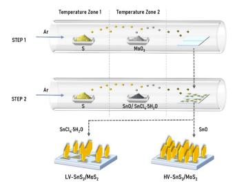
Fig. 1 Schematic of two-step direct vdW epitaxial growth of low densityvertical (LV) and high density-vertical (HV) SnS<sub>2</sub>/MoS<sub>2</sub> heterostructures.
