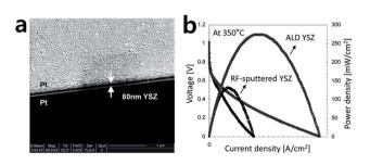
Fig. 4 (a) SEM image of ALD YSZ film between porous Pt cathode and anode. (b) Performance comparison of ALD YSZ fuel cells to fuel cells with 50 nm RF-sputtered YSZ. Figures reproduced with permission from ref. 37. Copyright 2007, American Chemical Society.
