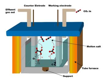
Fig. 1 Schematic of the MSCC-ET reactor.
