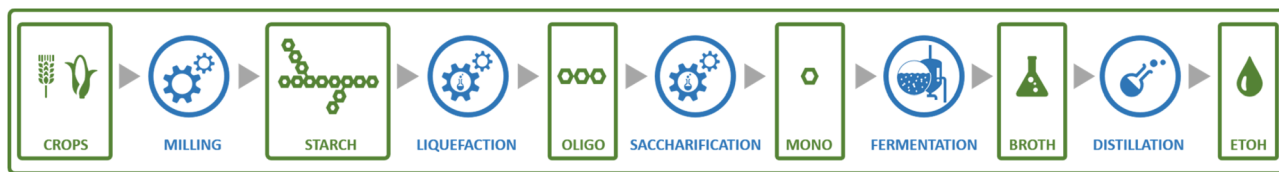
Fig. 2 Schematic representation of the steps involved in a typical process for the production of bioethanol from a first generation feedstock: corn starch.
