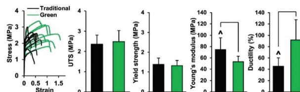
**Fig. 3** Comparison of the mechanical properties of membranes electrospun using green and traditional solvents. They performed similarly in ultimate tensile strength (UTS) and yield strength, while the elastic modulus was lower and the ductility higher for the green solvents. Reproduced from ref. 274 with permission from IOP Publishing.
