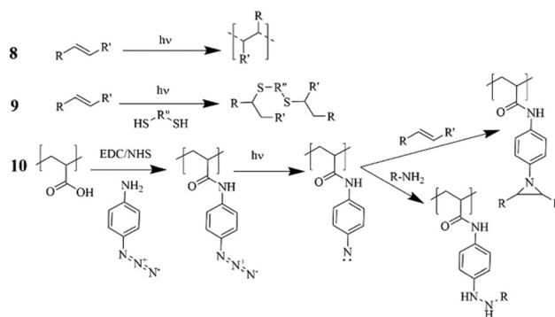
**Scheme 3** Overview of the different photo-induced cross-linking chemistries using (8) vinyl groups, (9) vinyl groups and thiols, and (10) polyacrylic acid and 4-azidoaniline forming nitrene intermediate under UV-light that can further react with amines or vinyl groups on polymers, thus acting as a cross-linker.
