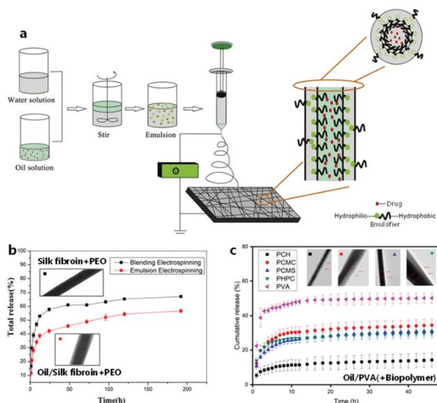
**Fig. 6** Principle and effect of electrospinning from emulsion for encapsulation purposes. (a) Schematic process of emulsion electrospinning. (b) Typical release profiles from emulsion-spun and blend-spun fibers including respective TEM images. (a and b) Adapted from ref. 85 with permission from Elsevier B.V. (c) Release profiles depending on different sheath materials including respective TEM images. Adapted from ref. 109 with permission from Informa UK Limited.
