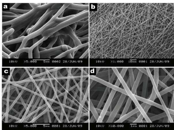
**Fig. 4** SEM images of (a) PAN fibers electrospun at 24 °C, and (b–d) Acyclovir-loaded PAN fibers electrospun at 80 °C with different magnifications. Reproduced from ref. 73 with permission from Elsevier.
