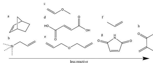
**Scheme 4** Chemical structure of molecules undergo photo-addition with thiols in order of reactivity: (a) norbornene, (b) vinyl silane, (c) vinyl ether, (d) fumarate, (e) allyl ether, (f) propene, (g) maleimide, and (h) methacrylate.
