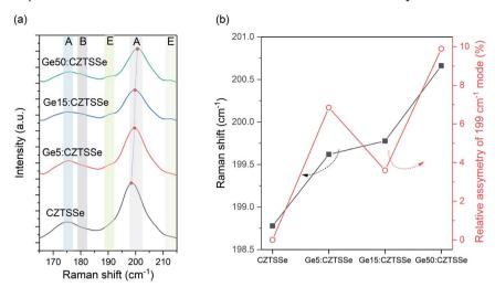
Fig. 4 (a). Raman spectra of CZTSSe films with or without Ge under 633 nm excitation. (b) Relative shift and asymmetry of the 199 cm<sup>-1</sup> peak measured for the CZTSSe films with and without Ge.
