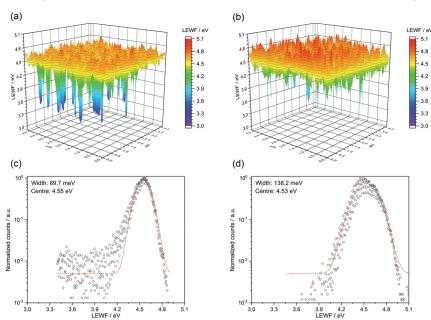
LEWF maps showing the electronic terrain for (a) CZTSSe and (b) Ge5:CZTSSe after a 500 eV Ar<sup>+</sup> plasma etching treatment. Affiliated LEWF distribution showing the spread of points for (c) CZTSSe and (d) Ge5:CZTSSe.
