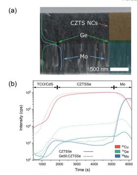
Fig. 1 (a) Elemental depth-profile of Ge and Mo acquired through an EDS lines scan overlaid onto a cross-sectional scanning electron micrograph of a CZTS precursor film. (b) SIMS depth profile of Ge, along with Cu and Mo, indicating the construction of the TCO/ CZTS/Mo structure upon annealing for CZTSSe and Ge50:CZTSSe.
