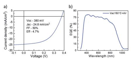
Fig. 4 (a) J-V characteristics and (b) EQE spectral response of the representative 4.7% efficiency device.
