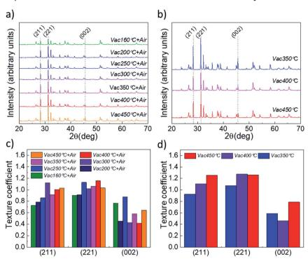
Fig. 6 XRD patterns of CSS  $Sb_2Se_3$  absorber films deposited at 460 °C onto  $TiO_2/FTO/g$ lass stacked substrates, with (a) vacuum and subsequent air annealed (Vac+Air)  $TiO_2$  and (b) vacuum annealed only (Vac)  $TiO_2$  layers. Related texture coefficients (TC) for (c) vacuum and subsequent air annealed (Vac+Air) and (d) vacuum annealed (Vac) films, calculated from the integrated intensity ratios (using the Harris formula<sup>46</sup>) for the dominant miller planes of  $Sb_2Se_3$ .
