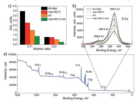
Fig. 7 (a) XPS survey spectrum of  $TiO_2$  films deposited by USP at 340 °C onto FTO/glass substrates. (b) C 1s core level from the as deposited (labelled as As-dep), 160 °C vacuum annealed (labelled as Vac160°C), 450 °C air annealed (labelled as Air), 160 °C vacuum and subsequent 450 °C air annealed (Vac160°C+Air)  $TiO_2$  films. (c) Calculated atomic ratios C/Ti and C/O for the related samples.
