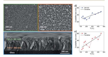
Fig. 2 (a and b) Top view SEM images of USP-deposited  $TiO_2$  after a 160 °C vacuum annealing step (Vac) and after 160 °C vacuum and subsequently 450 °C air annealing steps (Vac+Air), respectively. (c) Cross-sectional view of the  $TiO_2$  layer after 160 °C vacuum and subsequently 450 °C air annealing steps (Vac+Air). (d and e) Evolution of the crystallite size of vacuum and subsequently air annealed (labeled as Vac+Air) and vacuum annealed only (labeled as Vac)  $TiO_2$  films.
