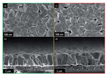
Fig. 5 Top-and cross-sectional view SEM images of CSS  $Sb_2Se_3$  absorber films deposited at 460 °C onto  $TiO_2/FTO/glass$  stacked substrates, with (a and b) 160 °C vacuum and consequent 450 °C air annealed  $TiO_2$  and (c and d) 450 °C vacuum and consequent 450 °C air annealed  $TiO_2$  layers.
