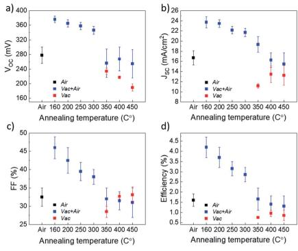
Fig. 3 J-V parameters, including (a) open-circuit voltage  $-V_{\rm OC}$ , (b) short-circuit current density  $-J_{\rm SC}$ , (c) fill factor - FF and (d) efficiency of  ${\rm TiO_2/Sb_2Se_3}$  devices with different  ${\rm TiO_2}$  annealing conditions.
