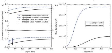
Fig. 3 (a) The VBM positions relative to the Fermi level,  $E_{\rm F}$ , determined by photoemission spectroscopy for Ag-doped and undoped GeSe (points) and the band bending profiles obtained by solving the Poisson equation (lines); (b) the hole density *versus* depth corresponding to the band bending profiles shown in (a).
