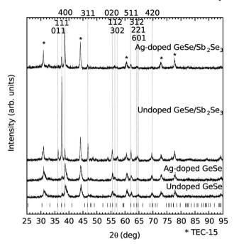
Fig. 5 Thin film XRD of the four film stacks along with the GeSe Bragg peak positions. Relevant Bragg peak positions are labelled and positions related to the SnO<sub>2</sub>:F coated substrate are starred.
