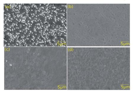
Fig. 4 Scanning electron microscopy images for devices (a) FTO/CdS/Ag:GeSe, (b) FTO/CdS/u:GeSe, (c) FTO/CdS/Sb<sub>2</sub>Se<sub>3</sub>/Ag:GeSe, and (d) FTO/CdS/Sb<sub>2</sub>Se<sub>3</sub>/u:GeSe, where Ag is the silver doped samples and u is undoped samples.
