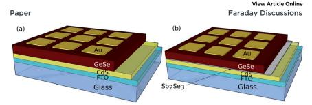
Fig. 1 The two different device structures investigated: (a) FTO/CdS/GeSe/Au and (b) FTO/CdS/Sb $_2$ Se $_3$ /GeSe/Au. Each device structure was made with both Ag-doped and undoped GeSe versions, making four device configurations in total.
