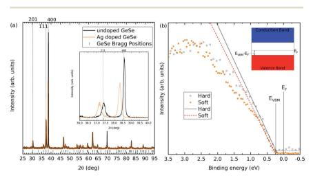
Fig. 2 (a) Powder XRD for undoped and Ag-doped materials. Bragg peaks for the 201, 111, and 400 reflections are shown with dotted lines. The inset shows the same data zoomed into the 111 and 400 peaks to highlight the shift in pattern. (b) The valence band measurements for the Ag-doped GeSe for hard and soft X-ray photoemission. The inset is a diagram explaining how the Fermi level position can be calculated using the signal onset.
