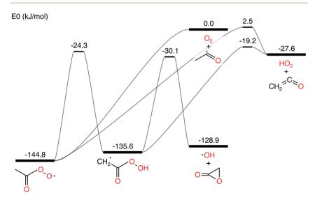
Fig. 1 Acetyl +  $O_2$  potential energy surface using parameters drawn from Allen et al. 2012.<sup>11</sup>
