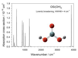
Fig. 2 Absorption cross section of OSi(OH)<sub>2</sub>, calculated at the B3LYP/6-311+g(2d,p) level of theory.
