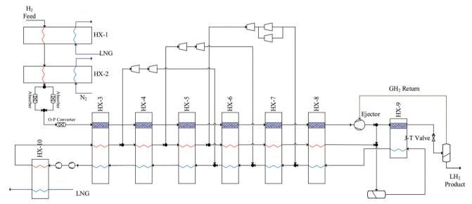
Fig. 9 Process block diagram for the Kuendig model. Simplifications have been implemented based on the original PFD: (i) N2 compressor system and N<sub>2</sub> cold box are combined as HX-2; (ii) H<sub>2</sub> compressor system is represented by HX-10; two individual cold streams through HX3-HX7 are combined as one cold stream.
