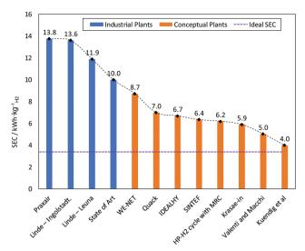
Fig. 11 Performance of industrial and conceptual hydrogen liquefiers. Feed and product conditions of ideal SEC calculation are: 1.01 bar, 303 K, 25% para-H<sub>2</sub>: 1.01 bar, 20 K, 99.8% para-H<sub>2</sub>. Purple dashed line corresponds to theoretical minimum.
