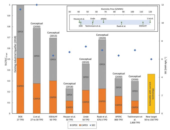
Fig. 14 Specific energy consumption (SEC) and specific liquefaction costs (SLC) relative to a reference 27 TPD LH<sub>2</sub> process (\$2.75 per kg H<sub>2</sub>) and the various conceptual processes estimated at different electricity costs
