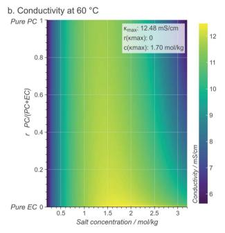
Fig. 4 Contour maps of electrolyte conductivity versus PC: EC molar ratio and conducting salt concentration, as predicted by our selected and trained model (egn.(3)) at (a) low and (b) high operating temperatures. The insets show the maximum conductivity and where is reached.
