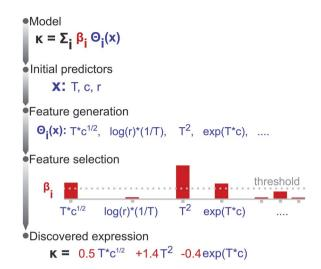
Fig. 1 Representation of the symbolic regression method. The conductivity  $\kappa$  is represented as a combination of non-linear operations applied on the original predictors: temperature T, conducting salt concentration c, and PC: EC molar ratio r. Based on multiple criteria, only few of the thousands of derived features are selected and used to build a 'discovered' expression.
