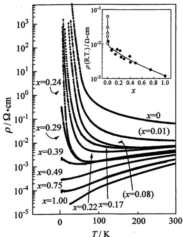
Fig. 5 Temperature dependence of the resistivity of  $(\text{DMDCNQI})_2\text{-Li}_{1-x}\text{Cu}_x$ . The inset shows the dependence of resistivity at RT with the white circles for the  $x = 0$  compound with various impurity levels. Reproduced from ref. 66. © 1999 The Physical Society of Japan.
