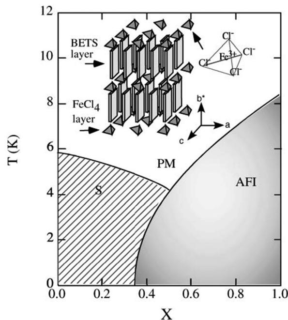
Fig. 7 Phase diagram of the organic alloys  $\lambda$ -(BETS)<sub>2</sub>Fe<sub>x</sub>Ga<sub>1-x</sub>Cl<sub>4</sub> in the absence of an external magnetic field. PM, AFI and S denote paramagnetic metal, antiferromagnetic insulator and superconductor, respectively. Reproduced from ref. 94. © 2003 The Physical Society of Japan.
