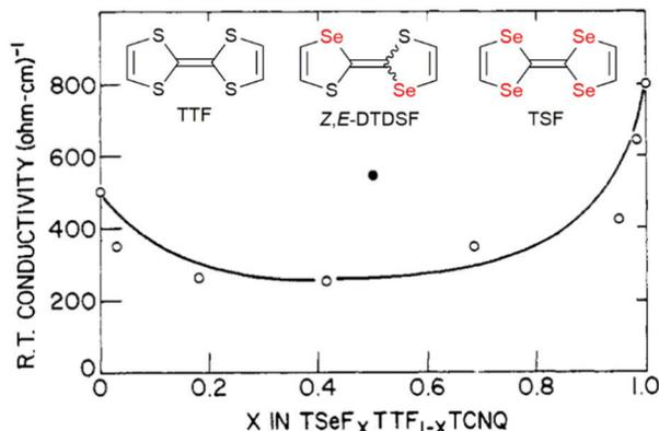
Fig. 4 Room temperature conductivity of  $(\text{TSF})_x(\text{TTF})_{1-x}(\text{TCNQ})$  (open circles). The closed black circle refers to  $[(\text{Z},\text{E})\text{-DTDSF}](\text{TCNQ})$  (see text). Adapted from ref. 34. © 1977 American Chemical Society.
