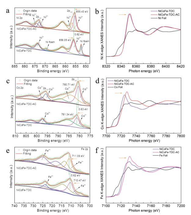
Fig. 3 Electronic structure characterization and mechanistic investigations of NiCoFe-TDC and NiCoFe-TDC-AC. (a) High resolution Ni 2p, (b) normalized Ni K-edge XANES spectra, (c) high resolution Co 2p, (d) normalized Co K-edge XANES spectra, (e) high resolution Fe 2p, and (f) normalized Fe K-edge XANES spectra
