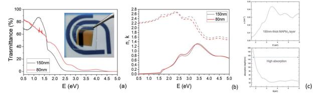
Fig. 7 (a) Transmittances of 150 nm and 80 nm MAPbl<sub>3</sub> films. (b) The refractive index n (dashed line) and the extinction coefficient k (solid line) of 150 nm and 80 nm MAPbl<sub>3</sub> films. Note the pre-gap tail that is close to ideality in the 150 nm-thick layer. (c) Absorption coefficient (nm<sup>-1</sup>) and absorption depth (nm) of 150 nm-thick MAPbl<sub>3</sub> layers.
