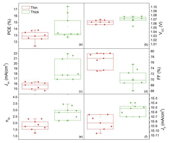
Fig. 10 Box plot of (a) efficiency (PCE), (b) open circuit voltage ( $V_{oc}$ ), (c) short circuit current ( $J_{sc}$ ), (d) fill factor (FF), (e) ideality factor ( $n_{iD}$ ) and (f) reverse saturation current  $(J_0)$  from the electrical characterization of all the prepared devices with 80 nm thick and 150 nm thick MAPbl<sub>3</sub> active layers.
