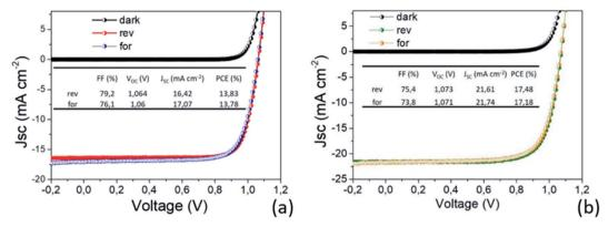
I-V characterization of the best prepared devices with (a) 80 nm and (b) 150 nm MAPbl<sub>3</sub> active layers. The AVT moves from 32.8% to 20%.
