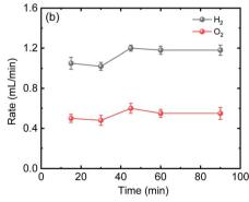
Fig. 2 (a) I-V curves of one (grey) and two 3J CPV cells (red) connected in series under 41-sun illumination overlapped with I-V curves of single (blue) and three (green) alkaline electrolysers connected in series. (b)  $H_2$  and  $O_2$  production rates from three alkaline electrolysers connected in series. Power is supplied from two CPV 3J cells connected in series under 41-sun illumination (without the use of Fresnel lenses to minimize further losses) as shown in Scheme 1.
