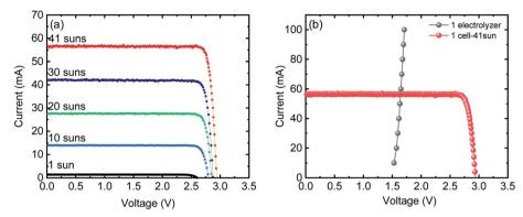
Fig. 1 (a) I-V characteristics of the InGaP/InGaAs/Ge 3J CPV cell (3 × 3 mm<sup>2</sup>) from Azur Space under one sun to 41-sun illumination (note the linearity of the current as a function of light concentration). (b) I-V curve of single alkaline electrolyser (grey) generated using CP measurements overlapped with the I-V curve of the 3J CPV cell (red) under 41 suns (without the use of Fresnel lenses).
