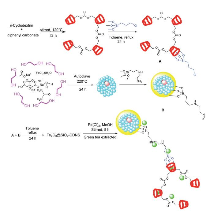
Scheme 57 The preparation of the Pd@h-Fe<sub>2</sub>O<sub>3</sub>@SiO<sub>2</sub>-CDNS.
