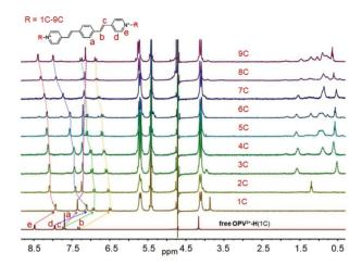
Fig. 3 <sup>1</sup>H NMR spectra of Q[8]/OPV<sup>2+</sup>-H (1C-9C) at a molar ratio of 2:2.
