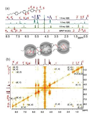
Fig. 4 (a)  $^{1}$ H NMR spectra of OPV $^{2+}$ -H (5C) (1.0 mM in D<sub>2</sub>O) with different concentrations of Q[8] (0-1.5 mM); (b) <sup>1</sup>H-<sup>1</sup>H NOESY of OPV2+-H (5C)/Q[8] at a molar ratio of 2:3.
