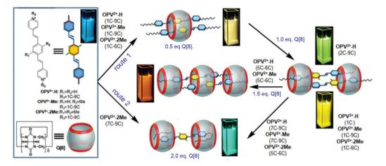
Scheme 1 Chemical structures of OPV<sup>2+</sup> derivatives and Q[8], and representation of Q[8]-based dynamic host-quest assemblies with multiple tunable fluorescence signals. Route 1: Q[8] concentration dependent host-quest interactions of 2:1, 2:2, 2:3, and 1:2 (quest/Q[8]); route 2: the formation of a U-shaped conformation of Q[8] with OPV<sup>2+</sup>-2Me (7C-9C).
