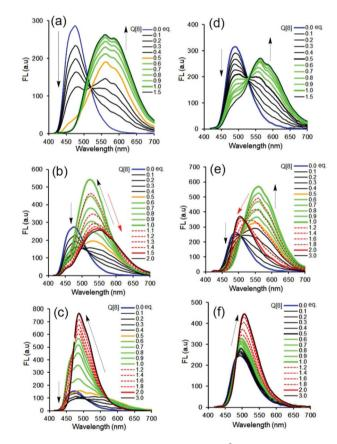
Fig. 1 Fluorescence spectrum changes of OPV<sup>2+</sup> core based guests (a– c) OPV2+-H (1C, 5C, and 9C), (d-f) OPV2+-2Me (1C, 5C, and 9C) (each of 10.0 µM in aqueous solution, pH 7.2) in the presence of increasing concentrations of the Q[8] host, respectively ( $\lambda_{ex}$  = 400 nm).
