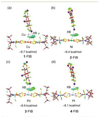
Fig. 9 Combined QTAIM and NCIplot surface analyses of 1-FIB (a), 2-FIB (b), 3-FIB (c), and 4-FIB (d) model clusters extracted from the X-ray coordinates. Bond and ring CPs are represented using red and yellow spheres, respectively. The color scale for the NCIplot is  $-0.03 < \text{sign}(\lambda_2)\rho < 0.03$ .
