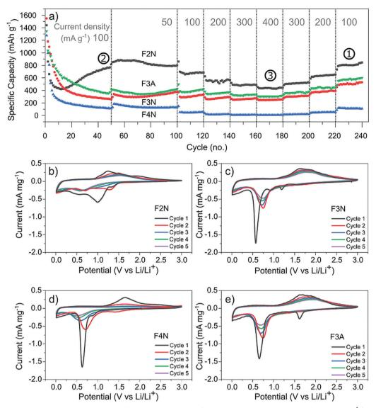
Fig. 4 (a) Discharge capacity of heat-treated samples (F2N, F3N, F4N and F3A) during galvanostatic cycling at 50-400 mA  $g^{-1}$  (relative to the active material mass). Specific capacities used for determining carbon content per Ah (Fig. 7) are indicated by the numbers (1, 2, and 3). (b)–(e) Cyclic voltammograms of (b) F2N, (c) F3N, (d) F4N and (e) F3A between 3.0-0.0 V vs. Li/Li<sup>+</sup> at a scan rate of 0.1 mV s<sup>-1</sup>.
