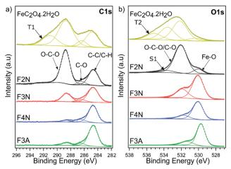
Fig. 2 High-resolution (a) C1s and (b) O1s XPS spectra for FeC<sub>2</sub>O<sub>4</sub>·2H<sub>2</sub>O, F2N, F3N, F4N and F3A. Spectra are vertically offset for clarity, and the deconvoluted components corresponding to key chemical groups are indicated. The component S1 is assigned as a satellite structure,  $^{40}$  and components labelled T1 and T2 tentatively assigned to CO2 and bicarbonate species
