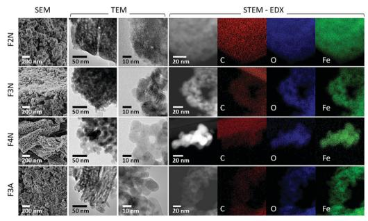
Fig. 3 SEM and TEM images showing the morphology of heat-treated samples (F2N, F3N, F4N and F3A). STEM-EDX elemental maps of FeC<sub>2</sub>O<sub>4</sub>·2H<sub>2</sub>O after heat treatment showing the distribution of C, O and Fe.
