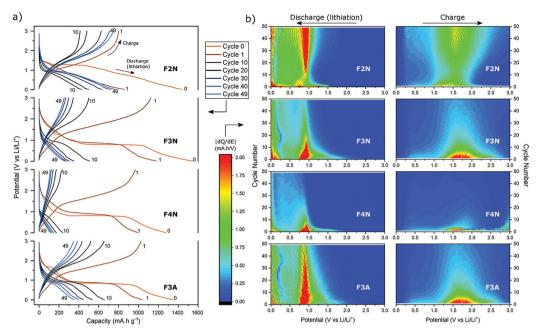
Fig. 6 (a) Potential profiles and (b) differential capacity maps of F2N, F3N, F4N and F3A galvanostatically cycled 50 times at 100 mA g<sup>-1</sup>. Differential capacity maps during discharge and charging show the changes to the charge and discharge capacity delivered at each potential as cycling progressed.
