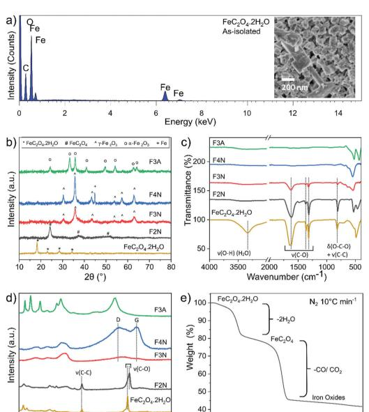
Fig. 1 (a) SEM-EDX spectral data and (inset) SEM image of as-isolated material. (b) PXRD patterns (c) FTIR spectra, (d) Raman spectra of as-isolated and heat-treated  $FeC_2O_4 \cdot 2H_2O$ , revealing chemical and structural changes after heat treatment. (e) Weight loss profile of as-isolated  $FeC_2O_4 \cdot 2H_2O$  during thermal decomposition in  $N_2$  (10 °C min<sup>-1</sup>).
