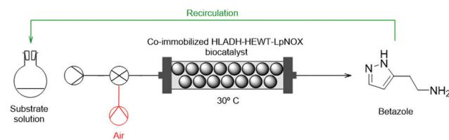
**Scheme 3** Continuous biocatalytic production of the betazole drug in a PBR. Substrate solution: 10 mM 2-(1*H*-pyrazol-3-yl)ethanol in phosphate buffer (0.05 M, pH 8), 1 mM NAD<sup>+</sup>, 20 mM IPA, 1 mM FAD, 0.1 mM PLP. T = 30 °C, P = atmospheric pressure. Reactor volume = 3.66 mL. In red: PBR implementing segmented liquid–gas flow composed of substrate solution/air. In green: PBR implementing recirculation of reaction solution (9.151 mL reaction solution volume).
