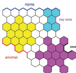
Scheme 3 Schematic representation of typical edge structures of PAHs.
