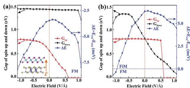
**Fig. 2** Electric field dependent band gaps of spin up (red) and down (black) states and total energy difference (blue) between the FM and FiM configurations for (a) the AB and (b) AC<sub>2</sub>' stacks.  $G_{\text{up}}$  and  $G_{\text{down}}$  indicate the band gaps in the spin up and spin down channel, respectively. As a matter of convention the electric field is positive when pointing from CrGeTe<sub>3</sub> to CrI<sub>3</sub>.
