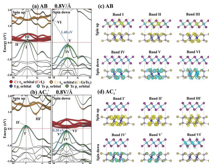
Fig. 3 Orbital-resolved band structures of the (a) AB and (c)  $AC_2'$  stacks under an external electric field of  $0.8 \text{ V \AA}^{-1}$ . Decomposed charge densities corresponding to the marked position of the bands for the (b) AB and (d)  $AC_2'$  stacking orders.
