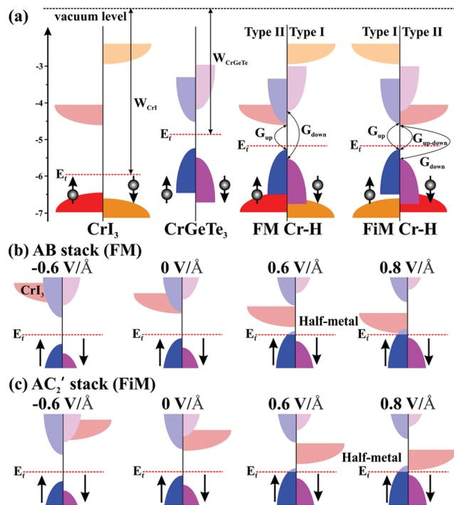
Fig. 4 Schematic band diagram for the (a) FM and FiM order and both (b) the AB and (c)  $AC_2'$  stacks under different external electric field. Only the bands near Fermi level are considered in (b) and (c). Red and Orange areas represent the valence band of  $CrI_3$  spin up and down channel, while Blue and pink areas are  $CrGeTe_3$  spin up and down channels, respectively. The corresponding light colors represent the conduction bands.
