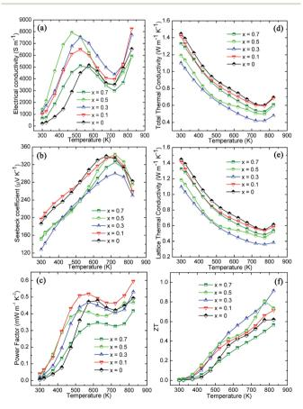
Fig. 8 Temperature-dependant thermoelectric properties of SnSe/ rGO-x (x = 0, 0.1, 0.3, 0.5, 0.7 wt%) pellets measured perpendicular to the pressing direction: (a) electrical conductivity, (b) Seebeck coefficient, (c) power factor, (d) total thermal conductivity, (e) lattice thermal conductivity, and (f) the figure of merit, ZT.
