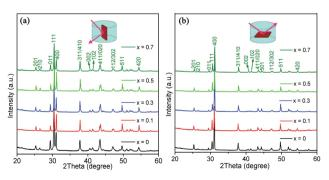
Fig. 5 XRD patterns of SnSe/rGO-x (x=0, 0.1, 0.3, 0.5, 0.7 wt%) sintered pellets measured (a) parallel and (b) perpendicular to the pressing direction.
