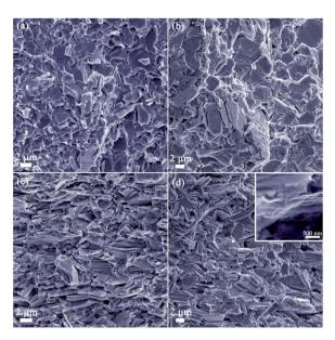
Fig. 6 Cross-sectional SEM images collected from fractured pellets (a and b) perpendicular and (c and d) parallel to the pressing direction for the sintered SnSe/rGO-x pellets: (a and c) x=0 wt%, (b and d) x=0.3 wt%. The inset in (d) is a magnified SEM image of part of the SnSe/rGO-0.3 pellet.
