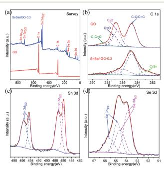
Fig. 3 XPS spectra of GO and SnSe/rGO-0.3 composite: (a) survey scan, (b-d) high-resolution scans for C 1s, Sn 3d and Se 3d, respectively.
