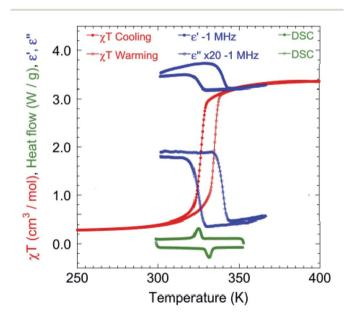
Fig. 3 Temperature dependence of  $\chi_M T$  in 1 kOe (red) at a rate of 2 K min<sup>-1</sup> (see Fig. S2† for the full temperature range of  $\chi_M T$ ), real and imaginary (×20) dielectricity (blue) at a rate of 20 K min<sup>-1</sup> and DSC (green) at a rate of 15 K min<sup>-1</sup> around the HS-LS transition.
