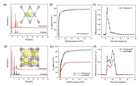
Fig. 2 The experimental and simulated PXRD patterns for compounds  $\bf 1$  (a) and  $\bf 2$  (d) after solvent removal. The  $N_2$  adsorption-desorption isotherms of compounds  $\bf 1$  (b),  $\bf 2$  and Ag NPs@2 (e) at 77 K. Pore size distribution of compounds  $\bf 1$  (c),  $\bf 2$  and Ag NPs@2 (f) calculated from  $N_2$  adsorption isotherms using a density functional theory (DFT) model.
