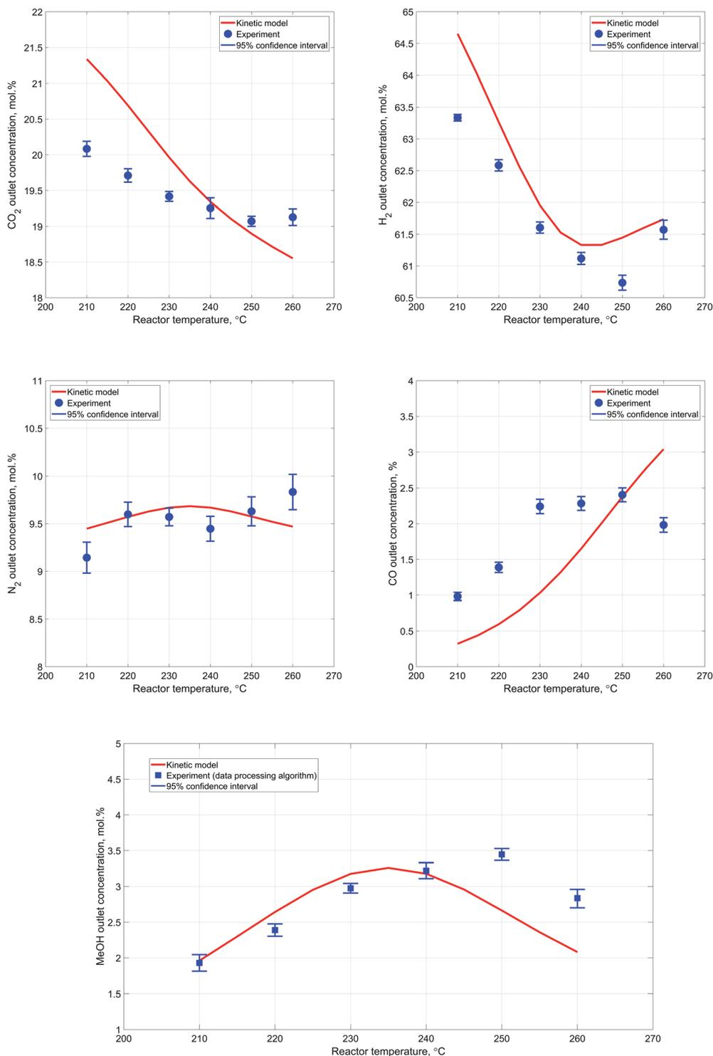
Fig. 8 (a). Dependence of the outlet CO<sub>2</sub> concentration from the reactor temperature. (b) Dependence of the outlet H<sub>2</sub> concentration from the reactor temperature. (c). Dependence of the outlet N<sub>2</sub> concentration from the reactor temperature. (d). Dependence of the outlet CO concentration from the reactor temperature.
