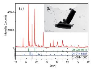
Fig. 3 (a) XRD pattern of anhydrous niobium oxide and the identified patterns. In the inset (b), a TEM image of the crystalline particles is shown (scale bar of 0.5 μm).
