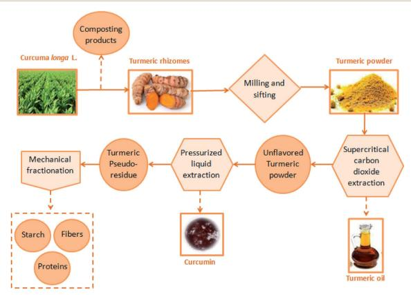
Fig. 2 Turmeric's biorefinery from clean emerging technologies.<sup>7,14</sup>
