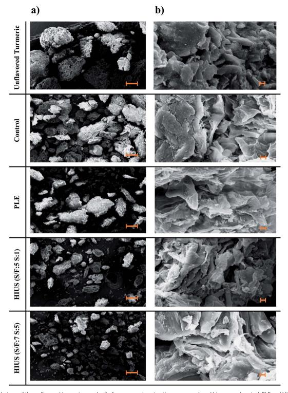
Fig. 9 Morphology of the unflavored turmeric powder (before curcumin extraction processes), and biomasses (control, PLE and HIUS). (a)  $250 \times (100 \ \mu m)$ , (b)  $5000 \times (2 \ \mu m)$ .
