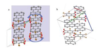
Fig. 1 Unit cell of perylene-TBPA in (a) HTP at 290 K and (b) LTP at 150 K. Curved arrows in (a) are included to highlight the TBPA dynamic reorientation. In TBPA the coloured atoms indicate oxygen (red) and bromine (brown). In the HTP of (a) the bromine and oxygen atoms appear superimposed because of the dynamical reorientation. The background plane in (a) represents the crystal face used for optical reflectivity measurements. Unit cell parameters are reported in the ESI.†
