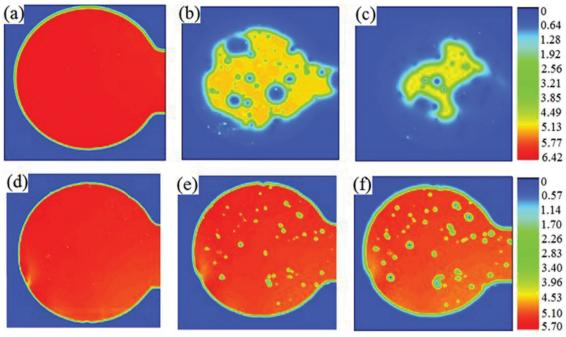
Fig. 5 Laser beam induced photocurrent images of the devices exposed to ambient air: (a and d) 0 days; (b and e) 4 days and (c and f) 8 days. The hole-transport layer was PEDOT:PSS (a-c) or  $MoO_3$ -PEDOT:PSS (d-f). The colour scale represents the photocurrent. Reproduced with permission.<sup>41</sup> Copyright 2013, WILEY-VCH Verlag GmbH & Co. KGaA, Weinheim.
