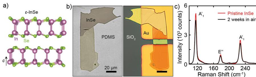
**Fig. 1** Layered semiconducting  $\epsilon$ -InSe. (a) Crystal structure of InSe. (b) Optical pictures of few-layer InSe exfoliated onto PDMS (left) and deterministically transferred onto pre-patterned gold electrodes (right). (c) Raman spectra (532 nm laser, power density  $0.11 \text{ mW } \mu\text{m}^{-2}$ ) of the InSe flake shown in panel b recorded in the pristine state and after two weeks in air conditions.
