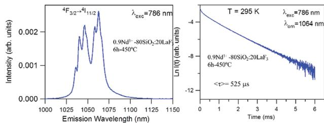
Fig. 9 Emission spectrum of 450 °C–6 h 0.9Nd<sup>3+</sup>–80SiO<sub>2</sub>:20LaF<sub>3</sub> sol and its corresponding semi-logarithmic plot of the experimental decay under excitation at 786 nm collecting the luminescence at 1064 nm.
