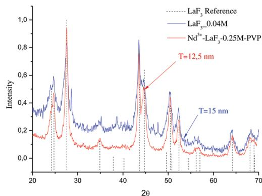
Fig. 2 XRD patterns of LaF<sub>3</sub>-0.04 and Nd<sup>3+</sup>-LaF<sub>3</sub>-0.25 M-PVP(10) nanoparticle suspensions dried at 80 °C for 12 h.
