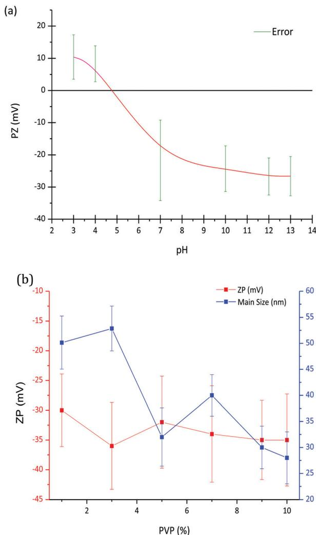
Fig. 1 (a) Variation of the ZP (mV) of LaF<sub>3</sub>-0.04 M nanoparticle suspensions as a function of pH and (b) variation of the zeta potential and particle size of LaF<sub>3</sub>-0.04 M nanoparticle suspensions at pH = 7 as a function of PVP wt%.
