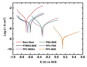
Fig. 4 PDP curves of bare steel and CPUDs-coated CS in 3.5 wt% NaCl solution for 3.0 h.
