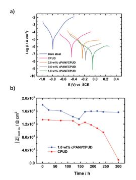
Fig. 6 (a) PDP curves for bare steel, pure CPUD and composite coatings in 3.5 wt% NaCl solution; and (b) plots of  $|Z|_{0.01 \text{ Hz}}$  against the immersion time for pure CPUD and the 1.0 wt% cPANI/CPUD composite coating
