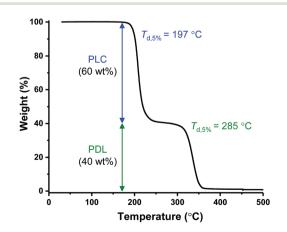
Fig. 2 Thermal gravimetric analysis data for ABA (87,60).
