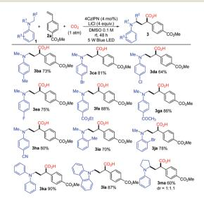
Scheme 3 Photocatalytic reactions of methyl 4-vinylbenzoate 2a with amines. Reaction conditions: 1 (1.2 mmol), 2a (0.2 mmol), 4CzIPN (0.008 mmol), LiCl (0.8 mmol), DMSO (2 mL), 1 atm CO<sub>2</sub>, 5 W blue LED, room temperature, 48 h, quenched with HCl (2 M) solution. Yields of isolated carboxylic acid 3 without esterification with TMSCHN2.
