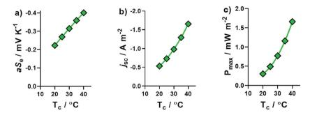
Fig. 4 Plots showing the significant effect different applied  $T_c$  values have upon the thermogalvanic properties of the  $[Fe(SO_4)_2]^{-/2-}$  system, as quantified by the (a)  $aS_e$ , (b)  $j_{SC}$ , and (c)  $P_{max}$ . For all measurements  $\Delta T = 10$  K, applied  $T_h = T_c + 10$  °C, and applied  $T_c$  is indicated by the x-axis. Second order polynomial lines of best fit have been added to guide the eye of the reader, and are not intended to model the data.
