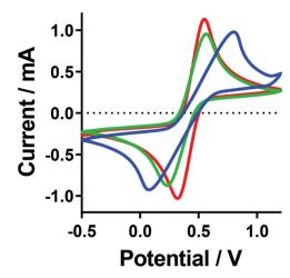
Fig. 7 Cyclic voltammagrams recorded for the  $[Fe(SO_4)]^{0/4}$  (blue line),  $[Fe(HSO_4)]^{1/2+}$  (red line) and  $[Fe(SO_4)_2]^{-/2-}$  (green line) systems. All recorded at ambient temperature using an Au working electrode, vs. an Ag/AgCl reference electrode, at 100 mV s<sup>-1</sup>. A table of data for the values can be found in the ESI.†
