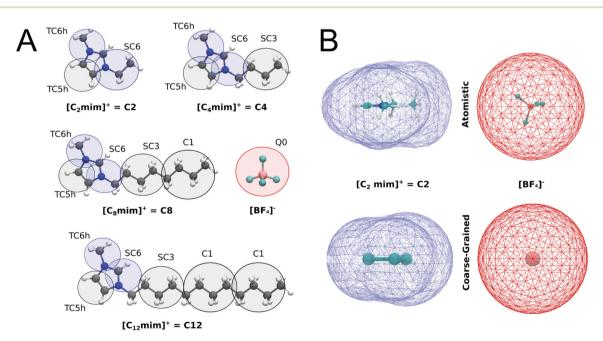
Fig. 1 Coarse-grain representations of imidazolium based ILs. (A) The Martini bead types and sizes of each bead are indicated. T and S prefixes mark the beads that use tiny and small beads. Blue and red colors indicate positively and negatively charged groups, respectively, while the gray color indicates the apolar groups. (B) Molecular surfaces (also called Connolly surfaces) of atomistic and coarse-grained structures of the C2 cation and the [BF4]<sup>-</sup> anion.
