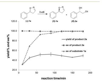
Fig. 2 Time course of the asymmetric ring-opening of 5-phenyl-4,5-dihydroisoxazole using Oxd B. The reactions were performed on a 500  $\mu$ L scale using 100 mM KPB buffer (pH 6.0), 1 U Oxd B, 20 mM 5-phenyl-4,5-dihydroisoxazole, 0.05 mM FMN, and 1 mM Na<sub>2</sub>S<sub>2</sub>O<sub>5</sub> at 30 °C. The yield and ee were determined using chiral HPLC (n = 2).
