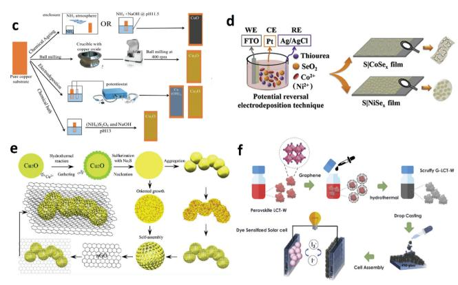
Fig. 12 Some of the most interesting and sustainable approaches to produce green and cost-effective counter-electrodes based on (a and b) waste-derived carbonaceous materials, (c and d) transition metal compounds and (e and f) composite materials. The figures have been adapted from ref. 321, 323, 345, 349, 337 and 358, respectively.
