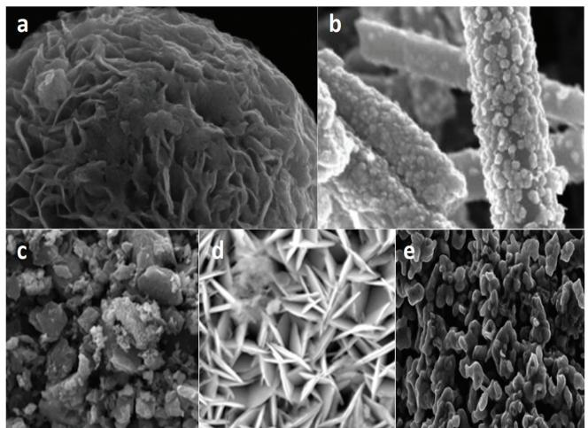
Fig. 11 Nanostructures of composite materials: (a) MoS<sub>2</sub>@rGO nanoflakes (adapted from ref. 355), (b) Ni<sub>3</sub>S<sub>4</sub> nanospheres supported on carbon nanotubes (adapted from ref. 357), (c) graphene-La<sub>2</sub>CdSnTiO<sub>4</sub>-WSe<sub>2</sub> nanopyramids (adapted from ref. 358), (d) hierarchical NiO@NiS@G nanocomposites (adapted from ref. 359) and (e) Ni/CoP<sub>x</sub>@CNTs nanostructures (adapted from ref. 360).
